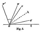
$\pi O \xi$  equals  $r \phi + s \theta$ ; or if the angle  $\sigma O \xi$  equals  $s \theta$  and the angle  $\pi O \xi$  equals  $r \phi$ , then the angle  $r O \xi$  equals  $r \phi - s \theta$ . Also, if the link  $O \pi'$  be fixed to  $O \pi$  (or O r) so as to make an angle  $\alpha$  with it, then the angle  $\pi' O \xi$  equals  $r \phi + s \theta \pm \alpha$  (or  $r \phi - s \theta \pm \alpha$ ).
